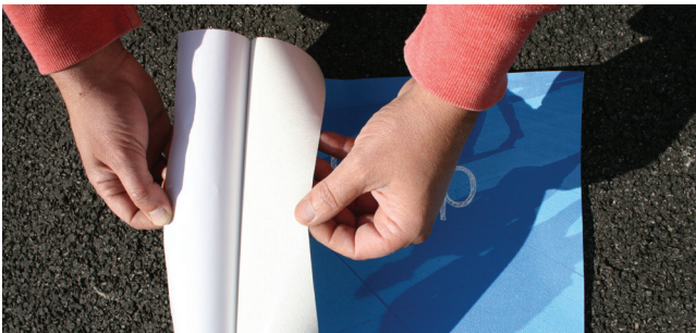
Remove a small amount of release liner from the surface for initial positioning purposes.
